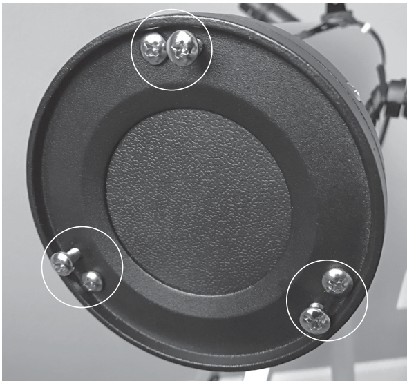
Figure 16. Align the primary mirror by adjusting the three pairs of “push/pull” screws on the back end of the optical tube.
