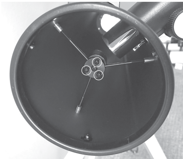
Figure 15. Adjust the tilt of the secondary mirror by adjusting the three alignment screws with a Phillips screwdriver.
