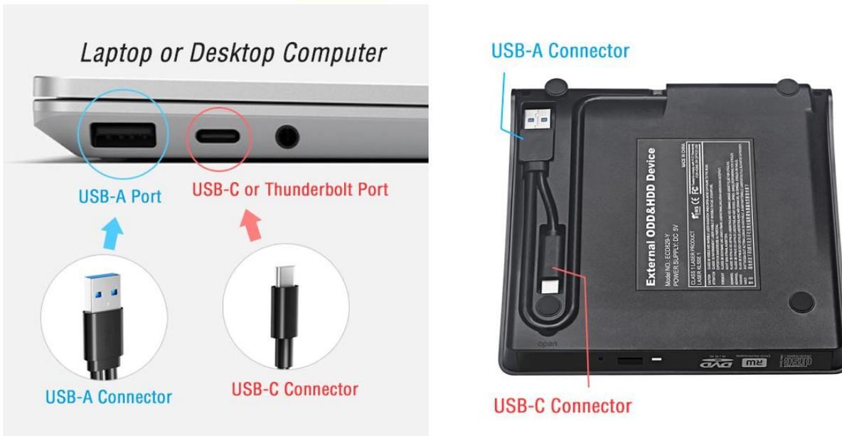
If the device you bought has extra power supply cord, we recommend you use it together with the data cable, which will ensure enough power, you can get extra power from a USB power adapter or another USB port on your computer.
